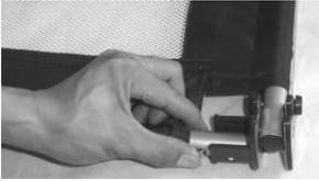
2. Press the spring button to unlock the tube.
